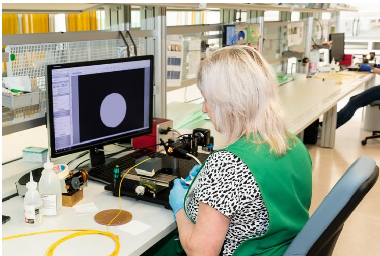
Image 3: Quality assurance through microscopic end face inspection. ©LWL-Sachsenkabel GmbH
