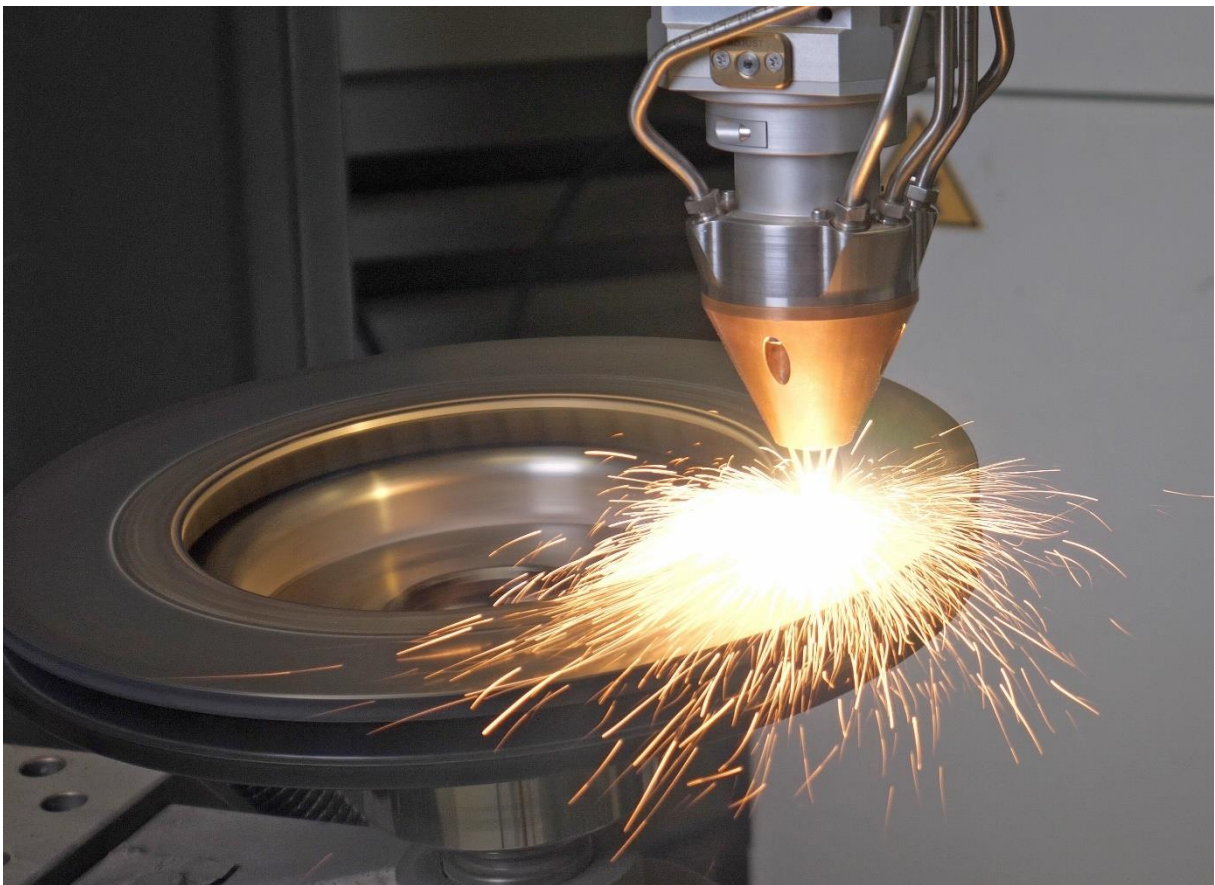
Figure 2: Powder-based laser coating of a brake disc. ©Laserline
