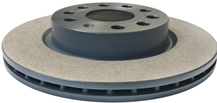
Figure 1: Brake disc following completion of the laser cladding. ©Laserline
