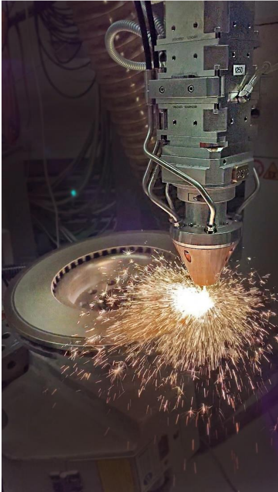
Figure 2: Powder-based laser coating of a brake disc. ©Laserline
